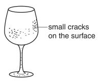
The cracks are caused by differences in the rate of diffusion of sodium ions and hydrogen ions in the glass.
