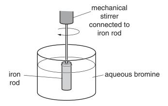
The iron is removed at regular intervals. It is washed, dried and then weighed. The iron is then replaced in the solution.
